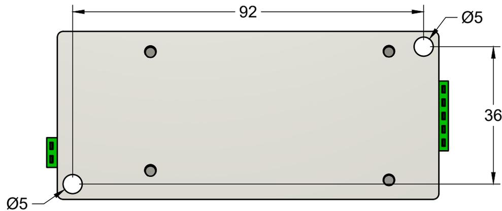
DRAWING DIMENSIONS APPLY TO EQUBE-P (1310-6000) AND EQUBE-N (1310-5000)
